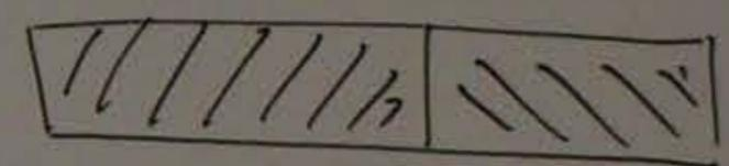
inf. bits      redundant (parity) bits
