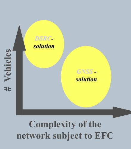
GNSS-solution: Very high flexibility when expanding the area; remote control of the geographical data and sections subject to EFC. Standard telecommunication components Enables advanced telematic services with additional value More expansive OBU
